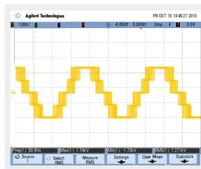
3-level output voltage waveform
