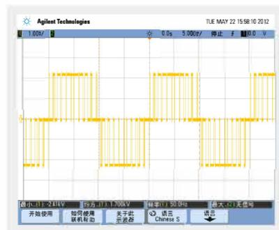
2-level output voltage waveform
